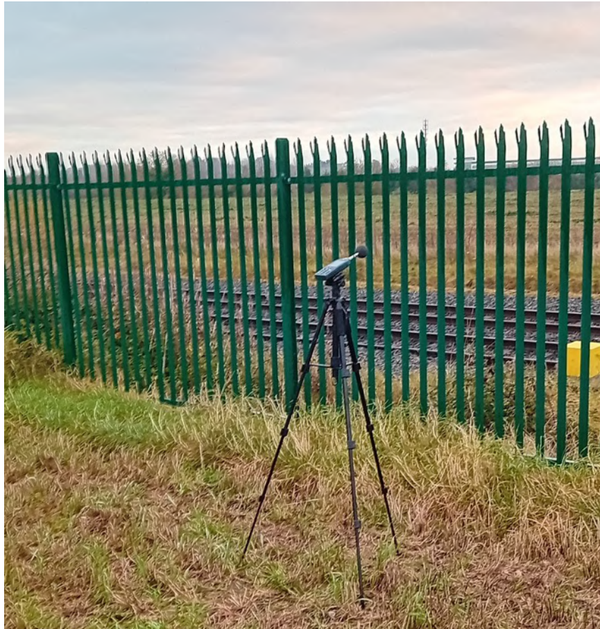
Figure 10.2: Attended Measurement Setup.
